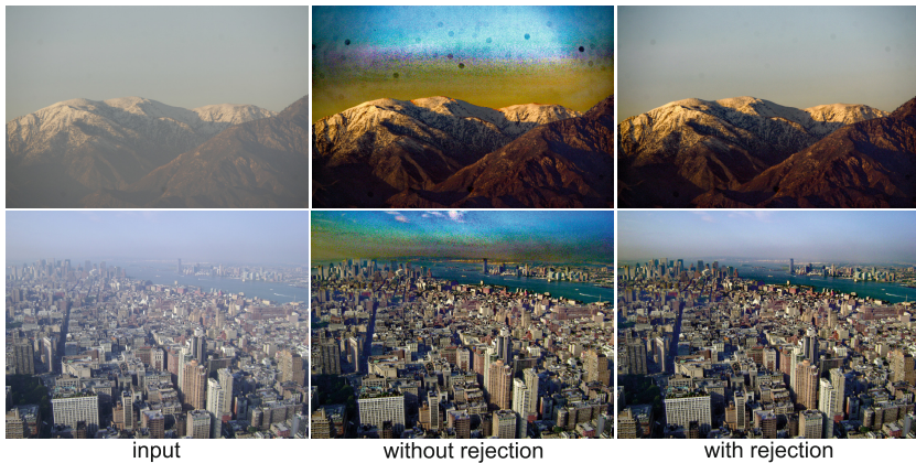
Fig. 14. Validation of our narrow angle outlier rejection method described in Sect. 3. In the second column, the distant region represented as sky has an infinite depth, and hence our transmission estimation stage estimates its transmission as being close to zero, which yields overly saturated results. We obtained consistent results by our outlier rejection stage, as shown in the third column. Images courtesy of Kim and Kim [1].
