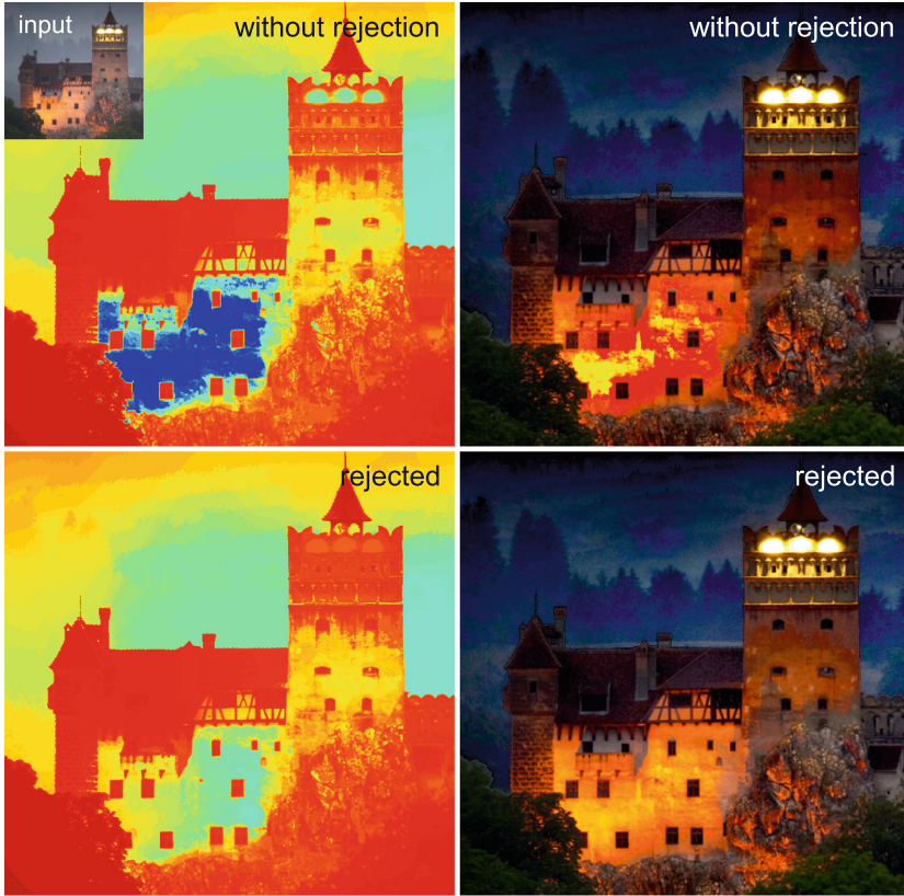
Fig. 15. Validation of our saturated outlier rejection method described in Sect. 3. The inset is an input hazy image. The first column shows estimated transmission maps without our rejection (upper left) and with our rejection (bottom left). The corresponding dehazed scenes are shown in the second column. The bright regions (the direct light at the upper right and the wall of the castle in the middle) are overly saturated. Our outlier rejection succeeds to produce a consistent result by discarding those regions.
