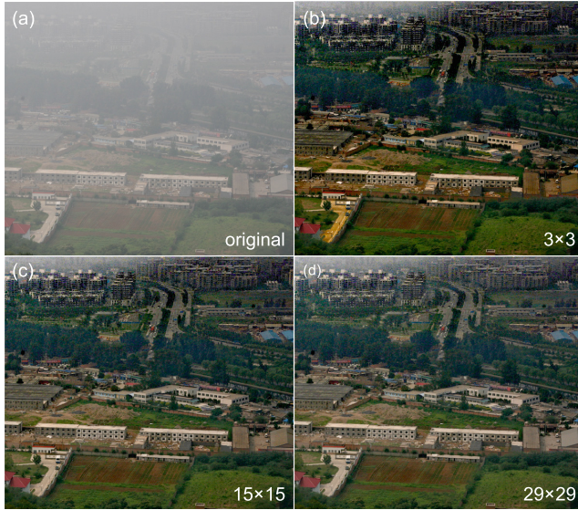
Fig. 13. Comparisons to show the influence of a patch size in estimating transmission. (a) The original canon image. (b) The dehazed image with a patch size of 3 \times 3 where severe color clamping happens. (c) The dehazed image with a patch size of 15 \times 15 , which is our choice for all results. (d) The dehazed image with a patch size of 29 \times 29 in which the airlight in distant regions is underestimated. Images courtesy of Kim and Kim [1].
